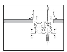
Do not screw too much to avoid damaging the gypsum. Screw to the right fit.
