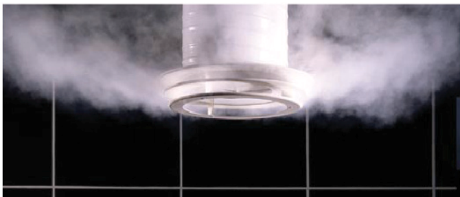
Radial stream - Cooling operation
