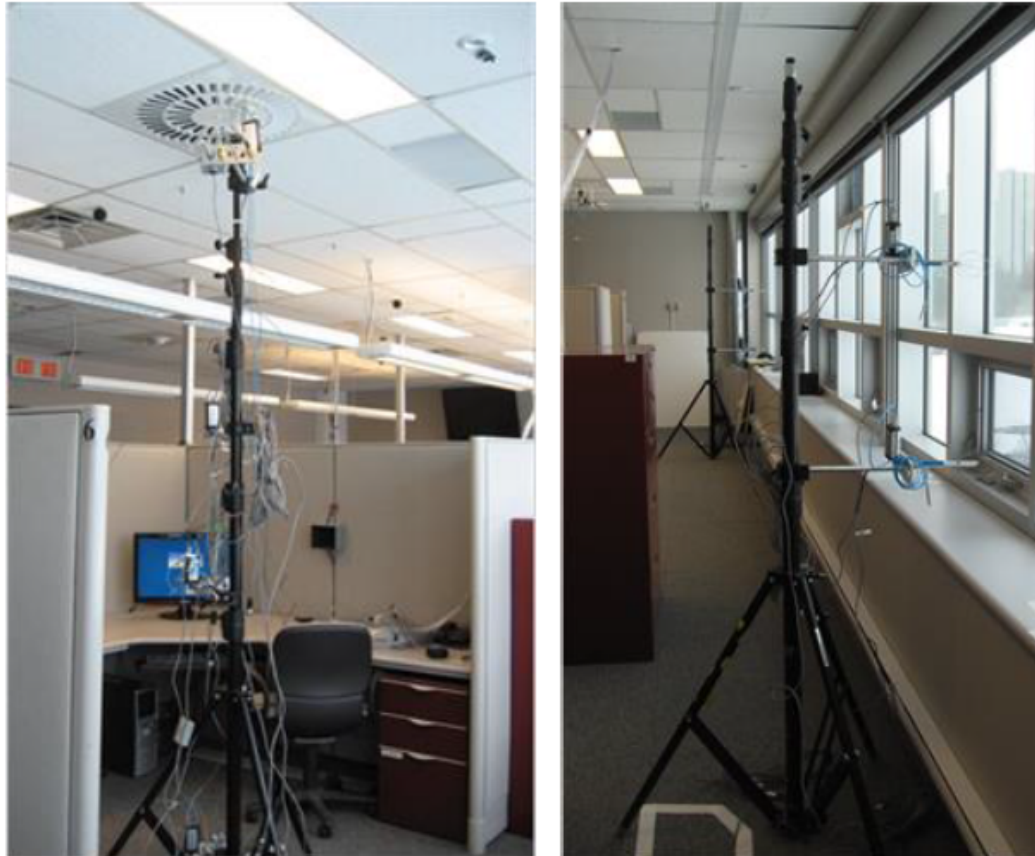
Figure 12: Measurement poles installed in a workstation (left) and at the exterior wall (window)
